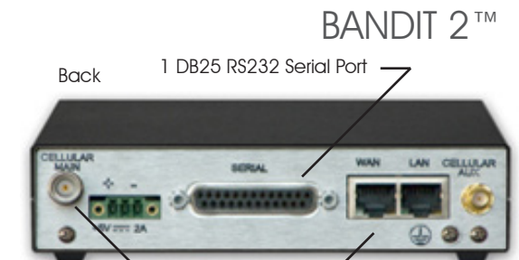
1 Optional Wireless Cellular and 2 10/100 Base TX Ethernet Ports
